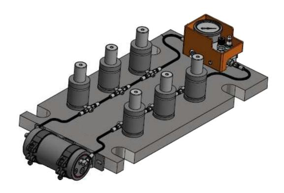
The Alfamak gas spring offers versatile functionality, allowing for independent or interconnected usage through appropriate connections. This enables precise force management and adjustment via a control panel, providing optimal balance for your specific requirements.
